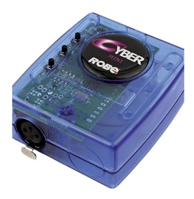
The Cyber Mini is the perfect product for small applications with less than 60 DMX channels. It offers a standalone memory with a maximum of 40 steps (60 channels) as well as 6 (4 + next/previous) ports for dry contacts triggering.
